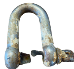
Steel shackle broken by metal corrosion due to the marine environment.
